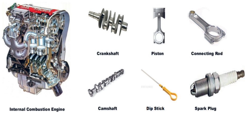
Fig. 1 wk8: Typical petrol engine and some major parts
